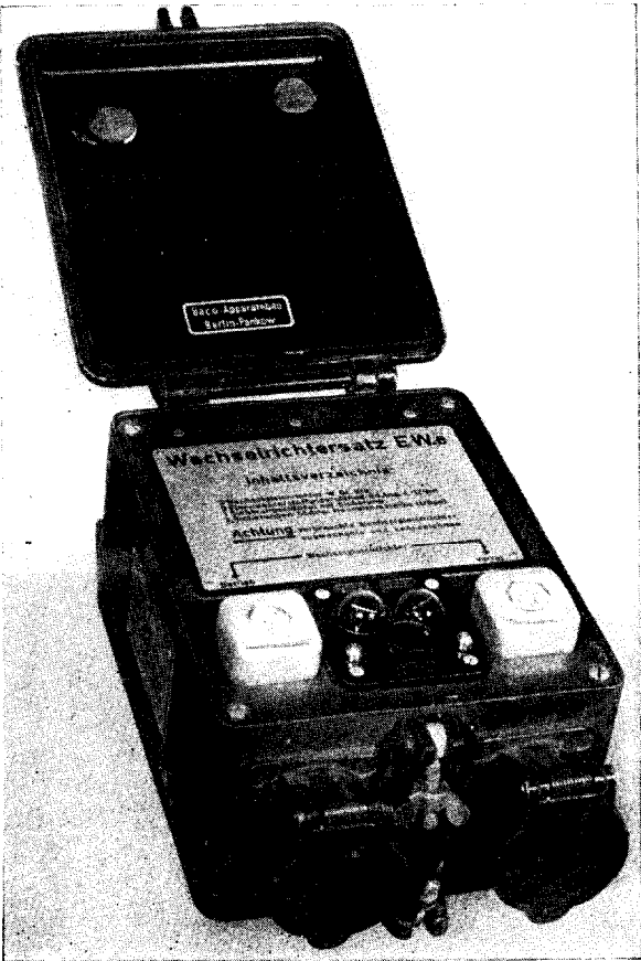
Figure 42.—Vibrator power supply EW.E.
