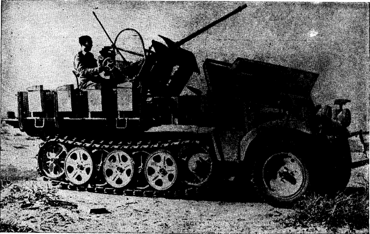
Figure 53.—2 cm Flak 30 (20-mm anti-aircraft gun) on half-track.
