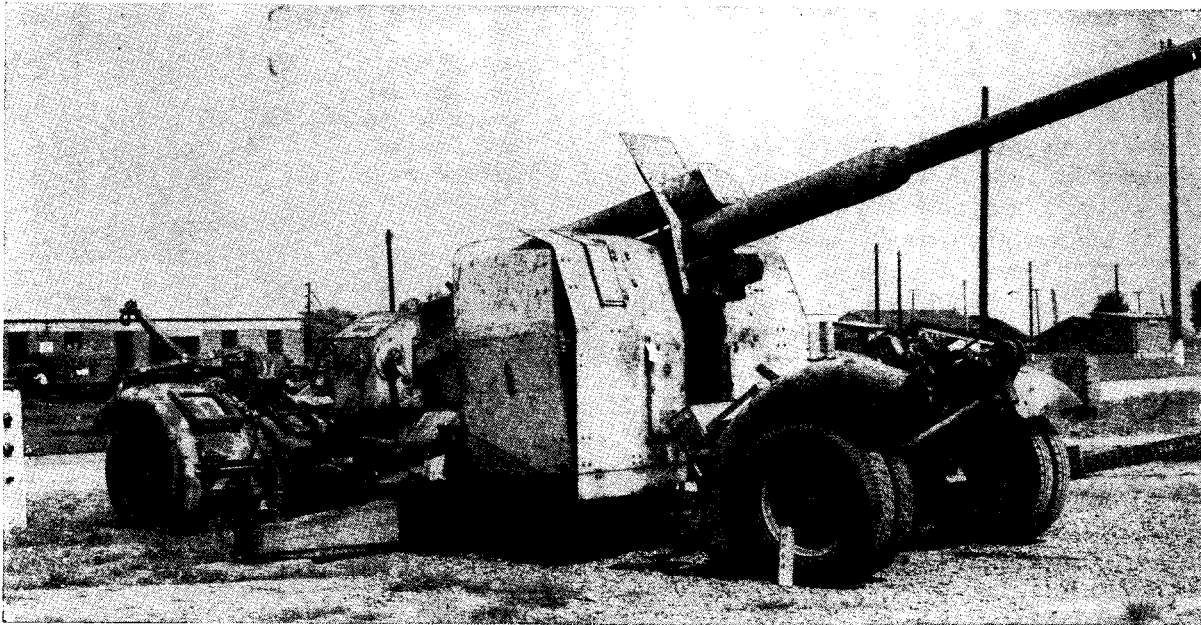
Figure 62.—8.8 cm Flak 41 (88-mm multipurpose gun) showing carriage lowered.
