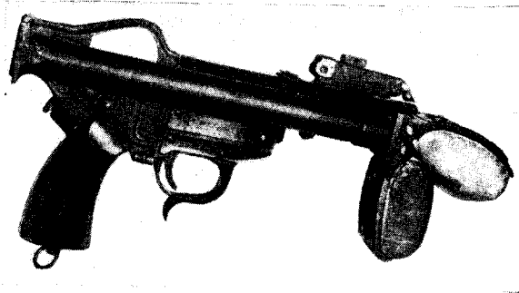
Figure 4.—Sturmpistole (modified light signal pistol).
