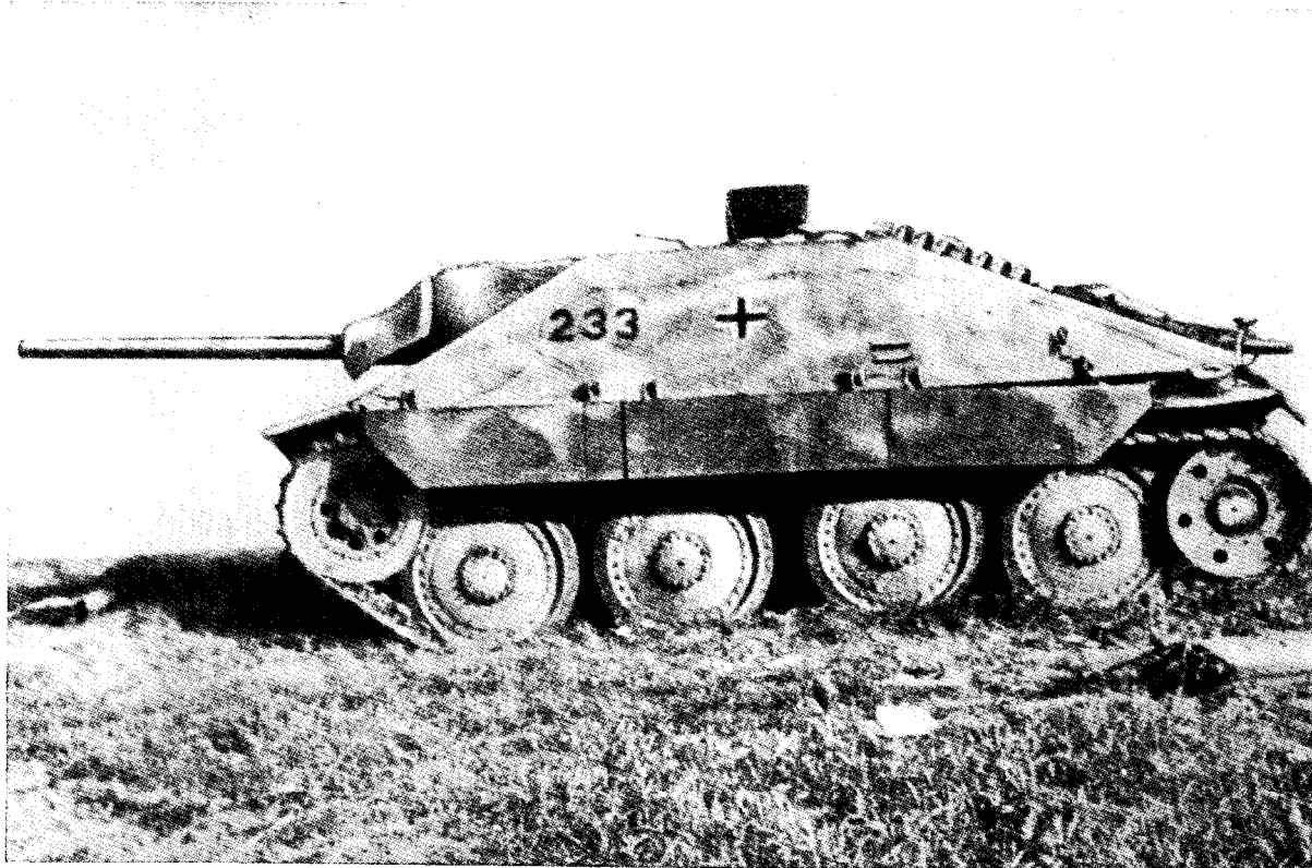
Figure 81.—7.5 cm Pak 39 (L/48) on Pz. Jäg 38.
