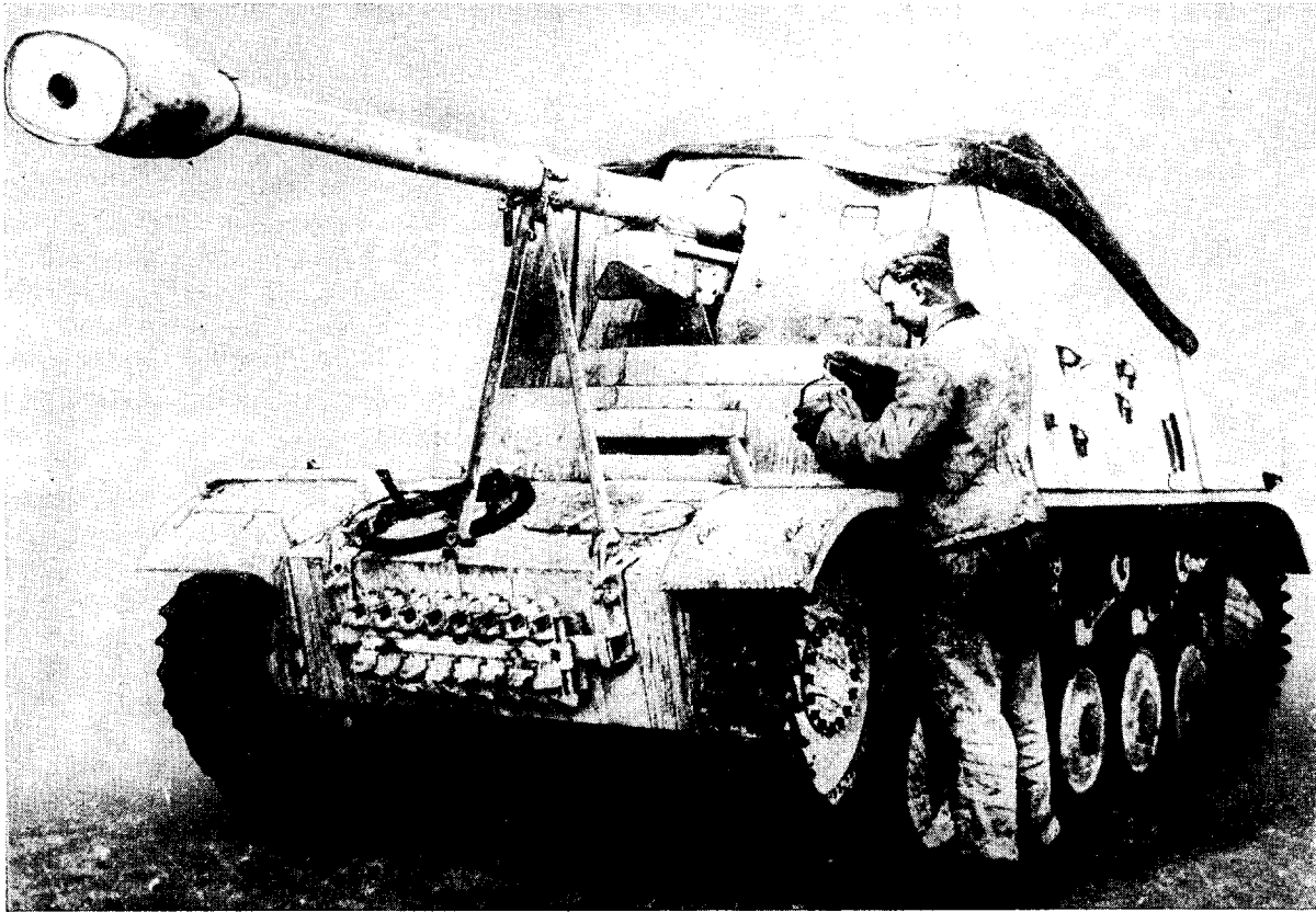
Figure 83.—7.5 cm Pak 40 on Pz. Kpfw. II Chassis.
