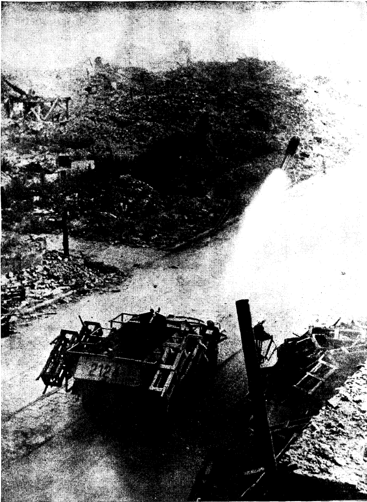
Figure 113.—The Wurfrahmen 40 is here shown in action. Four wooden rocket-carrying crates are in place on the plates on the side of the half-track. The last of the four rockets has just been fired. Empty crates lie at the right.
