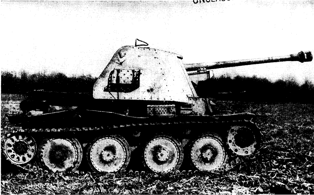
Figure 82.—7.5 cm Pak 40 on Pz. Kpfw. 38 (t) Chassis.
