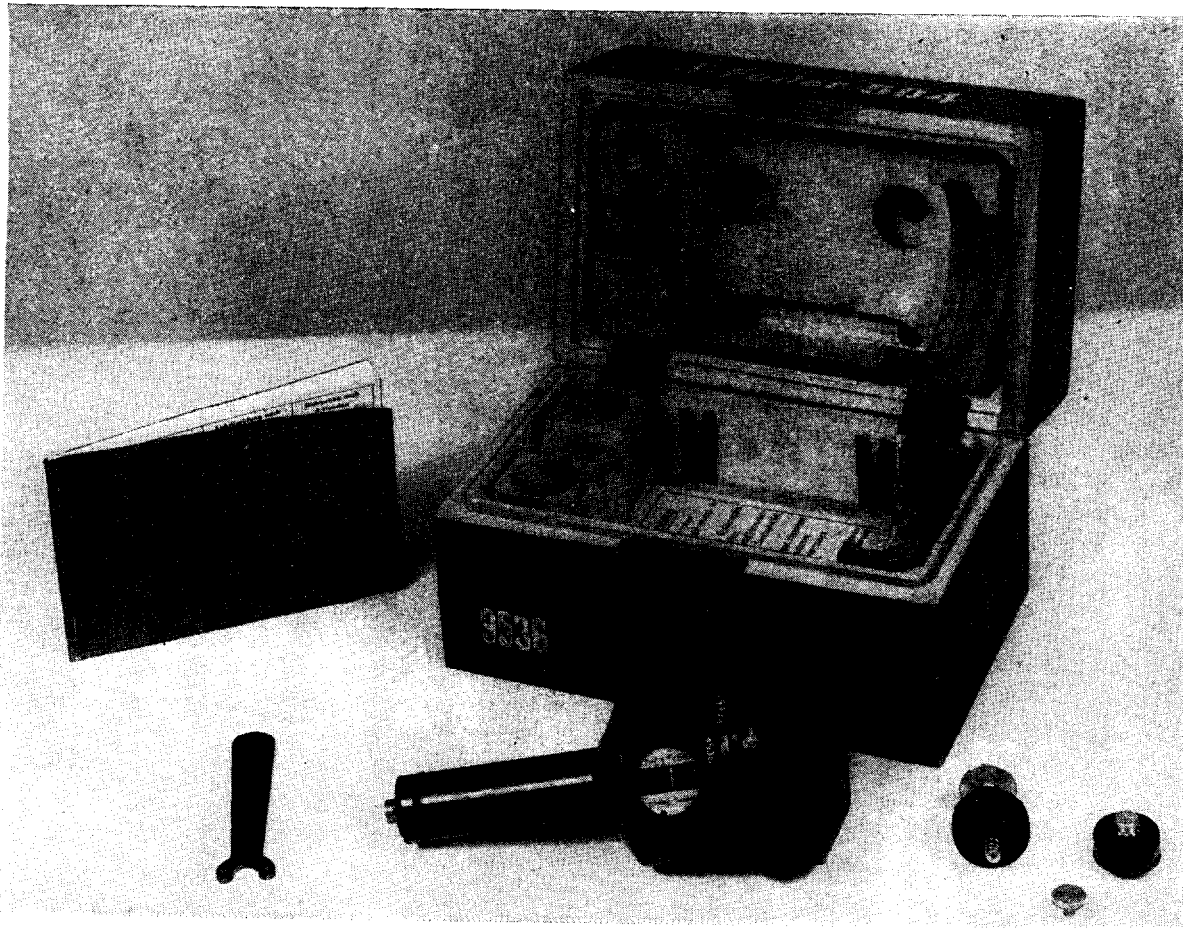
Figure 94.—Clockwork Long-delay Igniter (J-Feder 504).
